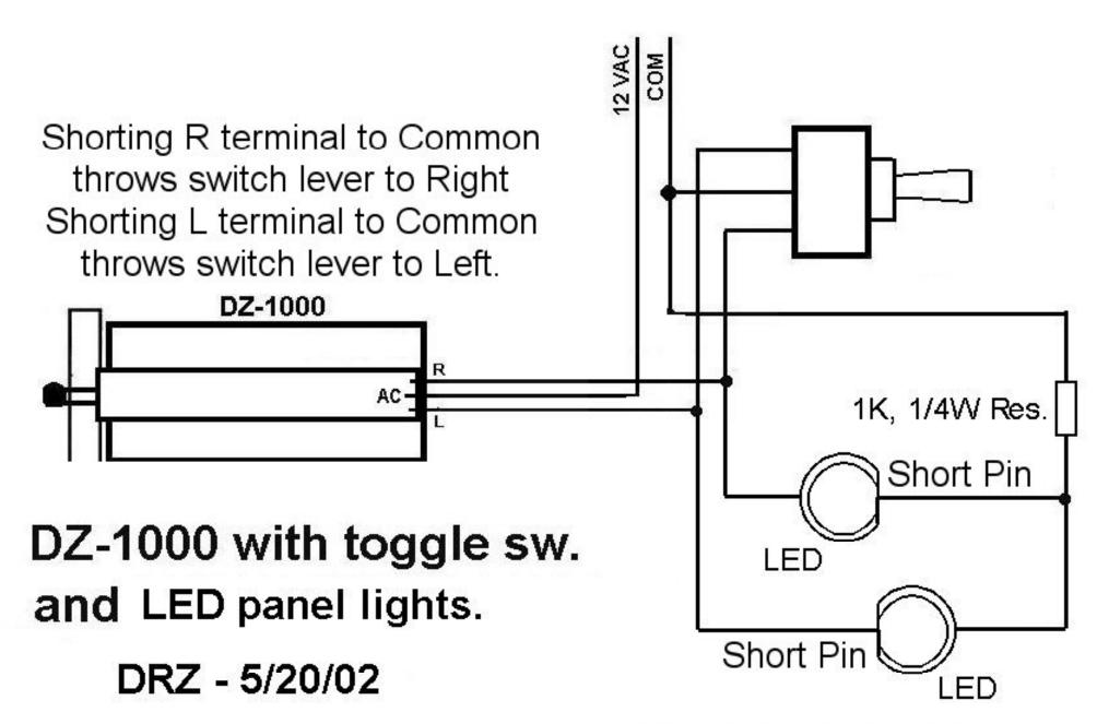
LEDs may need to be reversed for proper operation and indication.
